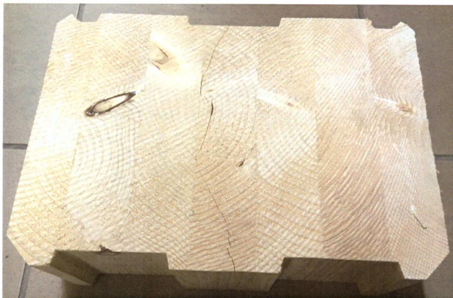
Picture 6. Damage of the sample LL/404/19/06
