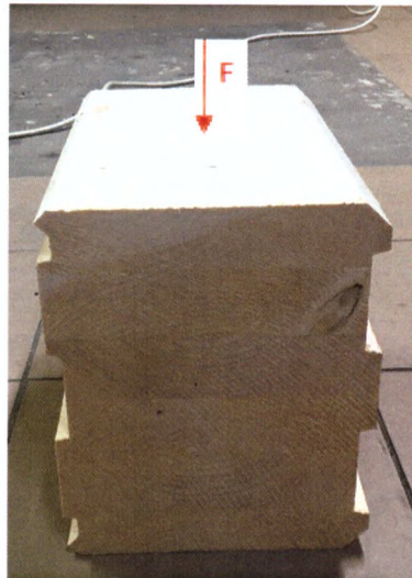
Picture 11. Method of loading the side surface of the sample
