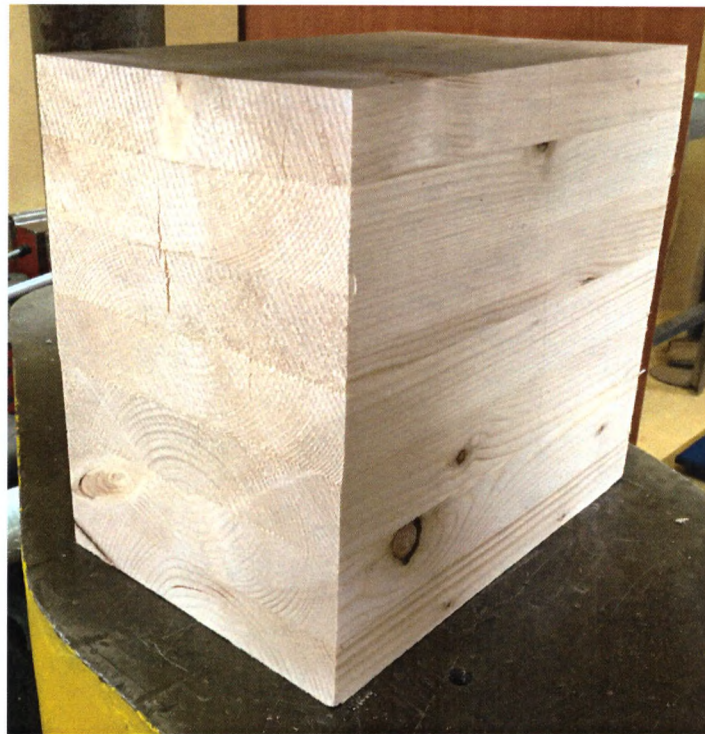
Picture 27. Damage of the sample LL/404/19/24
