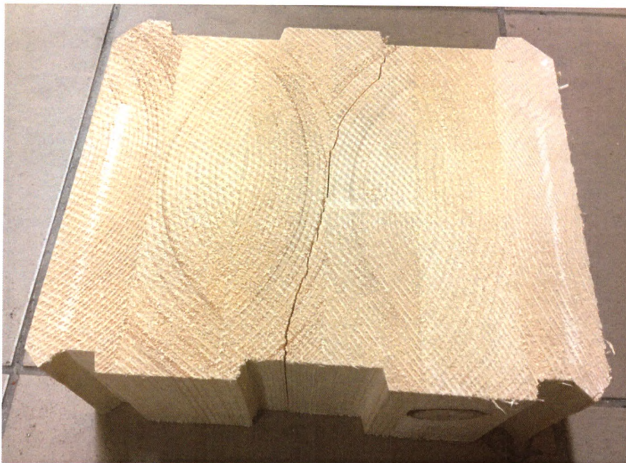
Picture 5. Damage of the sample LL/404/19/05
