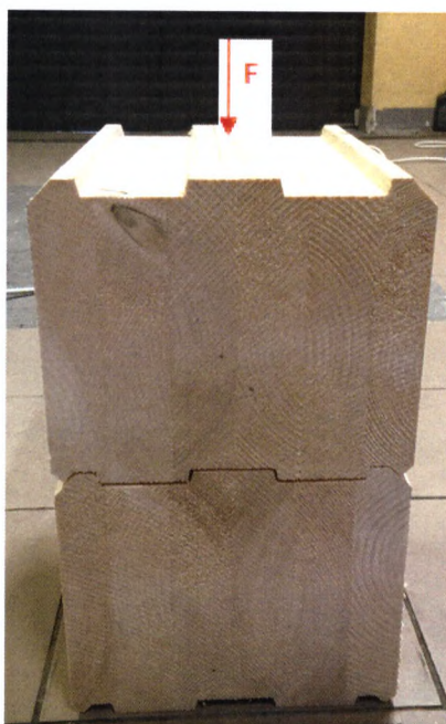
Picture 13. Method of loading the upper surface of two stacked samples
