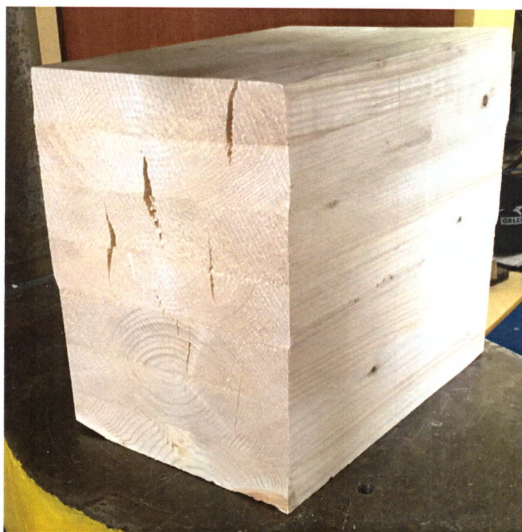
Picture 28. Damage of the sample LL/404/19/25
