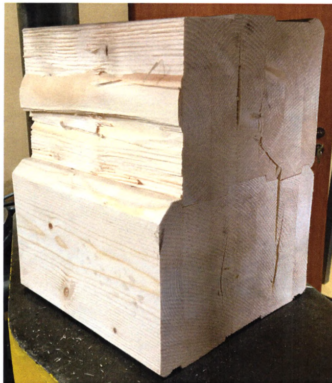
Picture 19. Damage of the sample LL/404/19/16
