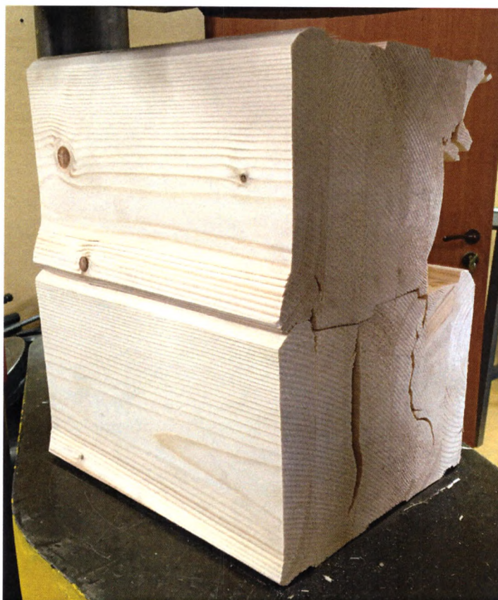
Picture 16. Damage of the sample LL/404/19/13
