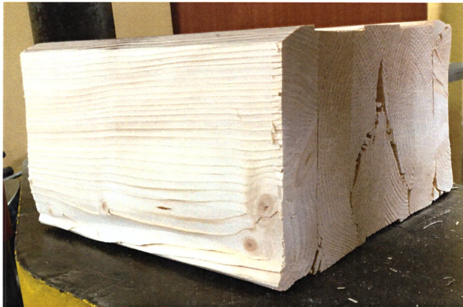
Picture 15. Damage of the sample LL/404/19/12
